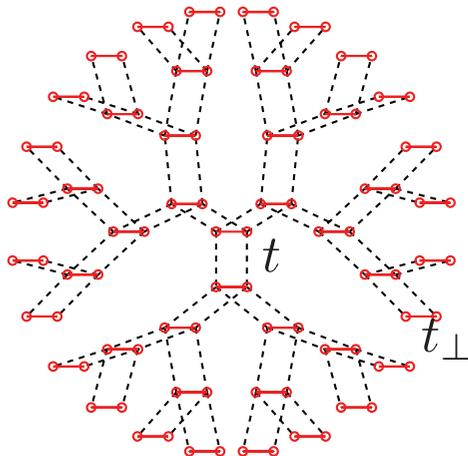
$$H = -t \sum_{\langle ij \rangle, \sigma} (a_{i\sigma}^{\dagger} a_{j\sigma} + b_{i\sigma}^{\dagger} b_{j\sigma}) - t_{\perp} \sum_{i\sigma} (a_{i\sigma}^{\dagger} b_{i\sigma} + b_{i\sigma}^{\dagger} a_{i\sigma}) + U \sum_{i\sigma} (n_{ai\uparrow} n_{ai\downarrow} + n_{bi\uparrow} n_{bi\downarrow})$$
